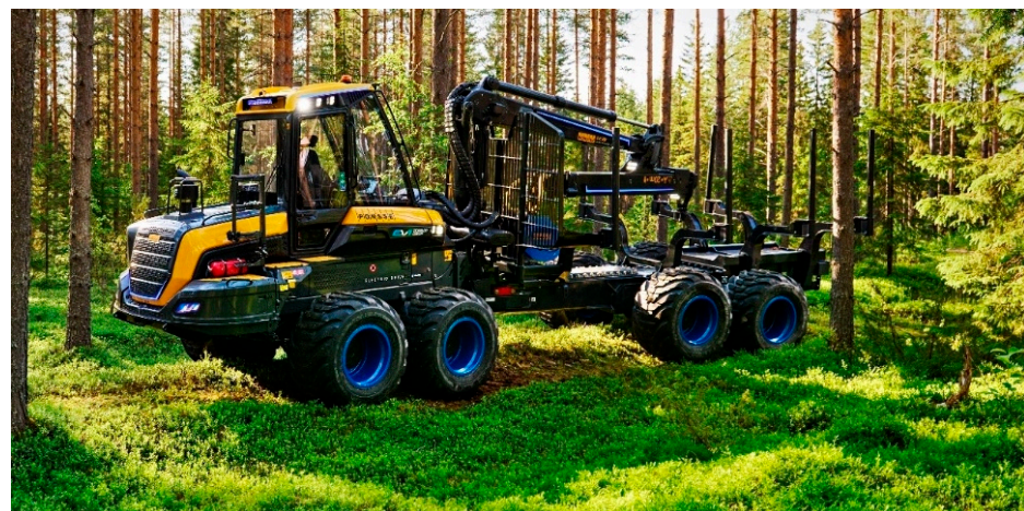
Figure 1. Ponsse EV1 electric series hybrid forwarder concept. Photo: Ponsse Plc.
